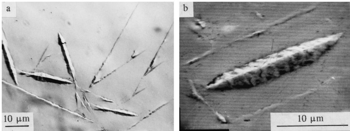
Fig. 1. Hydrogen-induced twins in the form of needles and deformation bands forming the surface relief of a ferritic steel single crystal (16% Cr). (a) Matrix orientation [111], magn. 1000 $\times$ ; (b) matrix orientation [100], magn. 3200 $\times$ .
