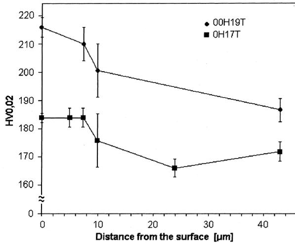
Fig. 4. Change of microhardness from the surface of the hydrogen-charged specimens of two ferritic stainless steels through their depth.
