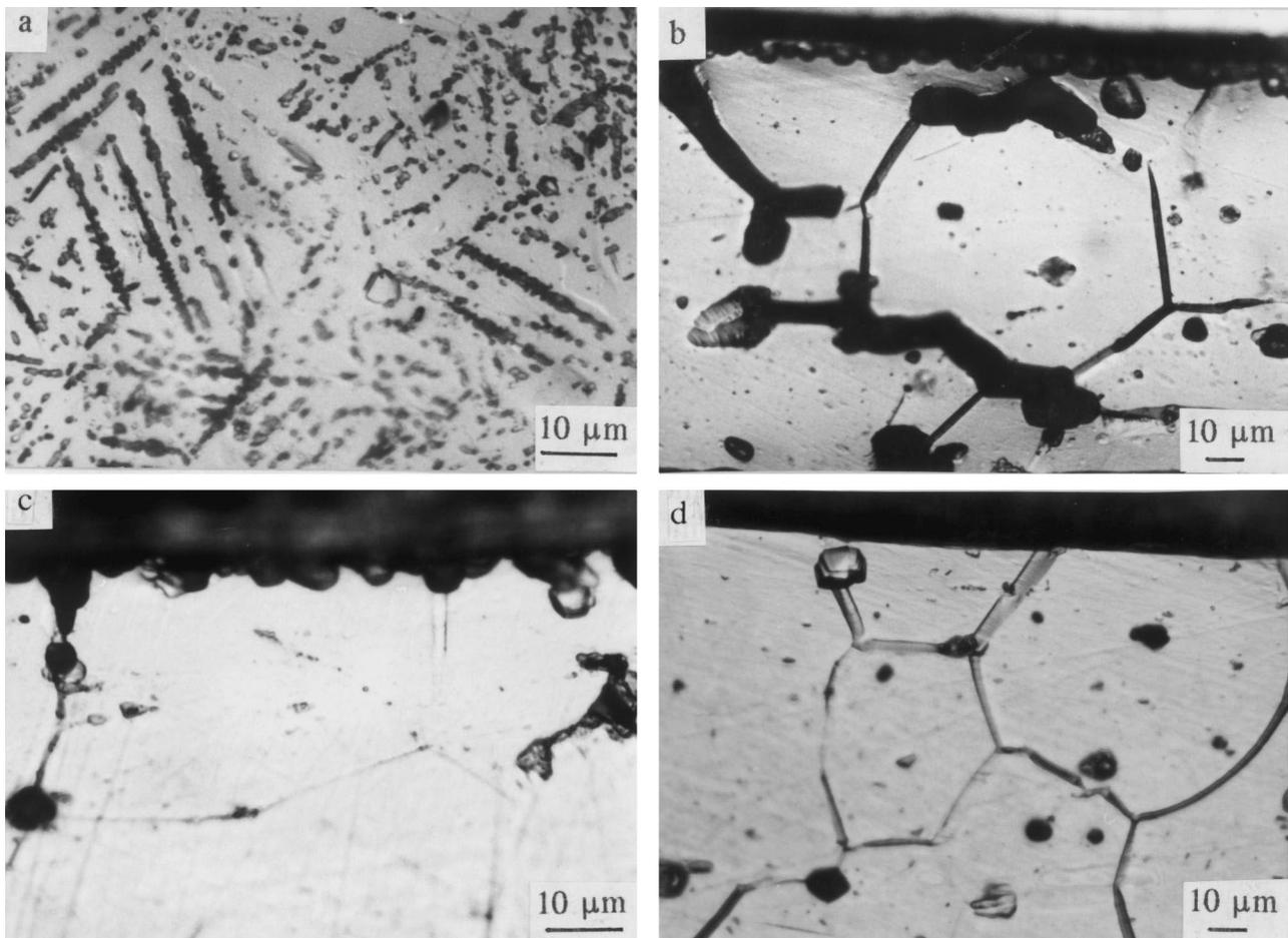
Fig. 2. Polycrystalline specimens of ferritic steel (19% Cr). (a) Hydrogen-charged and electrochemically etched surface of the sample, magn.1000 $\times$ . (b) Hydrogen-charged, cross-sectioned sample, mounted in a resin and electrochemically etched, magn. 500 $\times$ . (c) As in (b), magn. 1000 $\times$ . Notice a strong attack at the edge. (d) A cross-section of an uncharged specimen, mounted in a resin and electrochemically etched, magn. 500 $\times$ . Notice the smooth edge of the sample.
